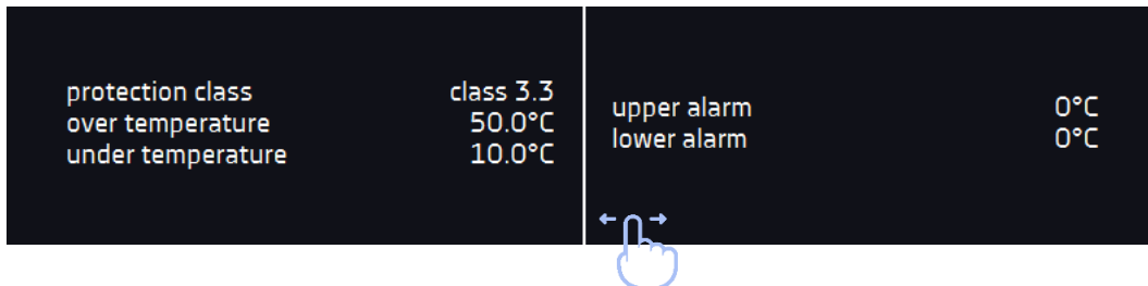
Figure 3 Status – protection and alarms
